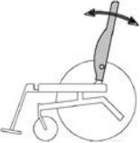
Lever for angle adjustment of the back support.
