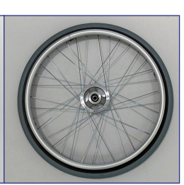
35 Flat free tires with drum brakes
