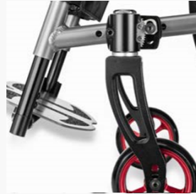
Individually adjustable chassis
