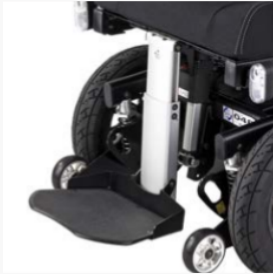
The central leg support makes a 90° knee angle possible
