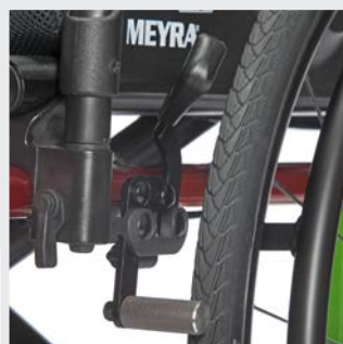
Unique brake with extremely low actuating force
