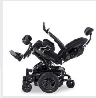
40° tilt for effective pressure relief
